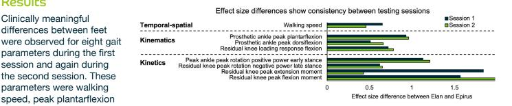
prosthetic ankle, residual knee loading response flexion, peak positive power during early stance at the prosthetic ankle, peak negative residual knee power during late stance, and peak stance phase extension and flexion moments at the residual knee. The mean effect size difference between foot types was similar over both sessions for each parameter, respectively.
